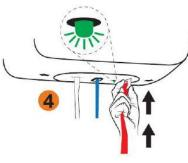
The white plastic tab must be pushed back into place in order to restore power to the lift.
