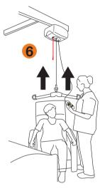
Never drag the lift along the track by pulling with the hand control.
