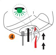
The white plastic tab must be pushed back into place in order to restore power to the lift.
