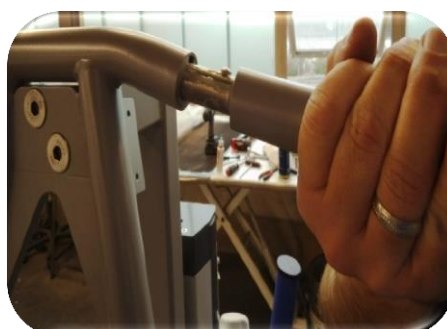
Picture 22: Now insert the safety arm into the seat socket. Make sure the two red markings face each other.
