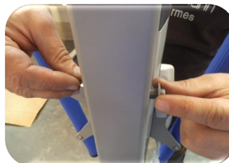
Picture 4: Now attach the washer from the other side.
