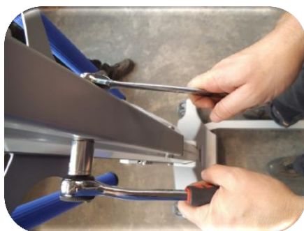
Picture 7: Now firmly tighten the screws using the ratchet and the box wrench.
