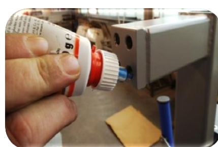
Picture 10: Now apply the new screw locking varnish to all 4 screw threads.
