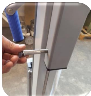
Picture 3: Attach the new seat socket to the lifter and insert the 2 screws from one side.
