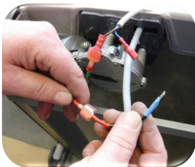
Picture 9.1: Remove the cable plug connectors from the motor.
