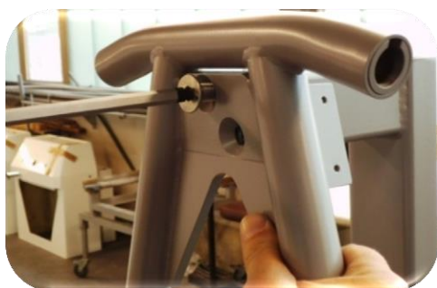
Picture 13: Now lightly tighten the screw into the seat.
