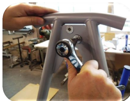
Picture 18: Firmly tighten the bottom screw and make sure that the seat stays in position.
