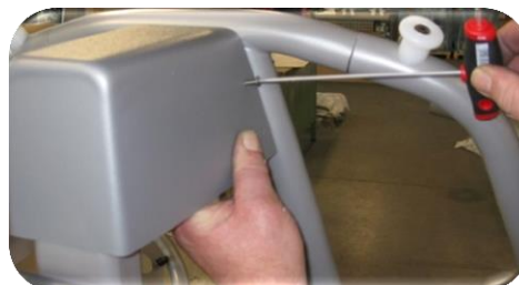
Picture 10: Now you can attach the seat cover with all 4 screws.
