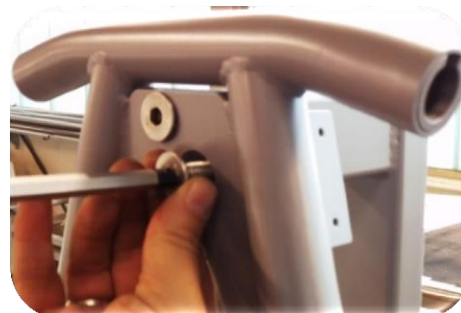
Picture 14: Now lightly tighten the screw into the seat.
