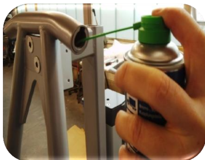
Picture 21: Also spray some Turbo Grease on the counterpart for taking in the safety arm.
