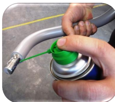
Picture 20: Before attaching the safety arms to the seat, Turbo Grease has to be applied on them.
