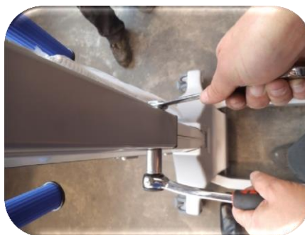
Picture 6: Now firmly tighten the screws using the ratchet and the box wrench.
