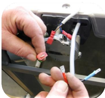
Picture 9.3: Remove the cable plug connectors from the motor.
