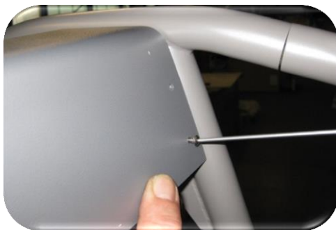
Picture 8: After marking, remove the safety bolt.
