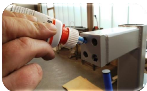
Picture 11: The screw locking varnish must be at least medium strong (21 Nm).
