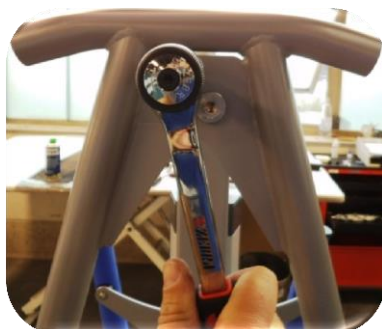
Picture 17: Firmly tighten the top screw and make sure that the seat stays in position.
