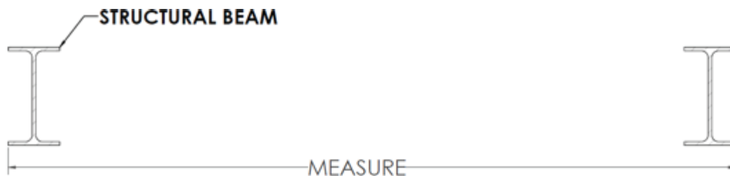
Figure 279: Measure Distance Between Structural Beams
