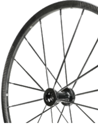
RW07 ↑ Spinergy CLX Carbon Blade*
