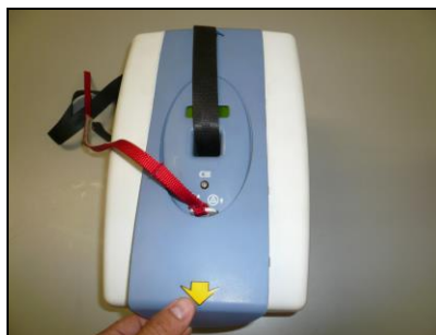
Detach bottom cover at one short side tab
