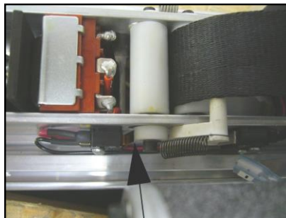
Bend the limit switch strip to ensure activation
