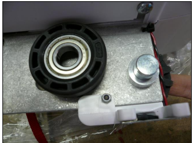
Remove & replace wheel from shaft
