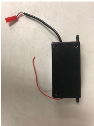
3 rd Generation Remote Relay Box with seat sensor wire and antenna
