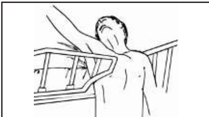
Zone 5 – Entrapment between split bed rails
