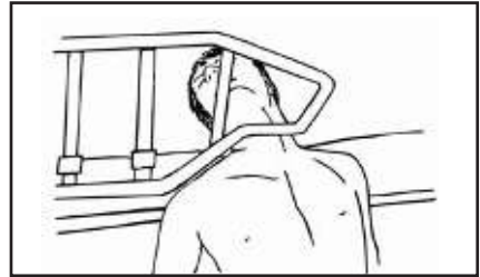
Zone 4 – Entrapment under the rail, at end of rail
