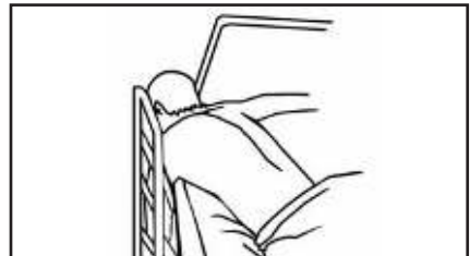
Zone 6 – Entrapment between the end of the rail and the side edge of the head or foot board
