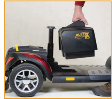
Step 2: Pull out the battery pack!
