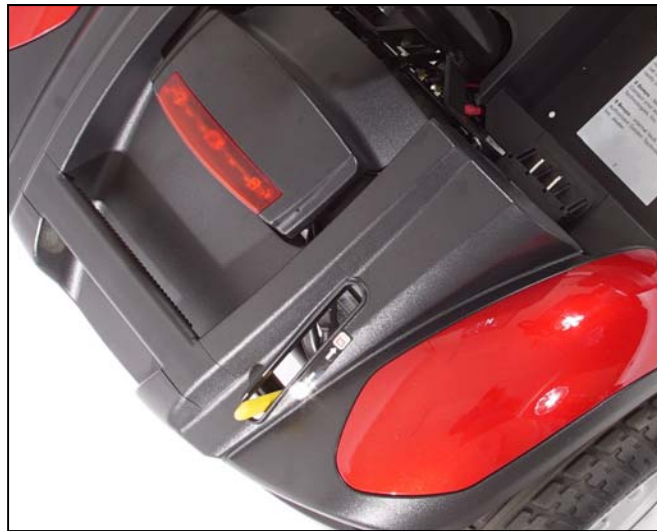
Figure 11: Freewheel Lever (Drive Position)
