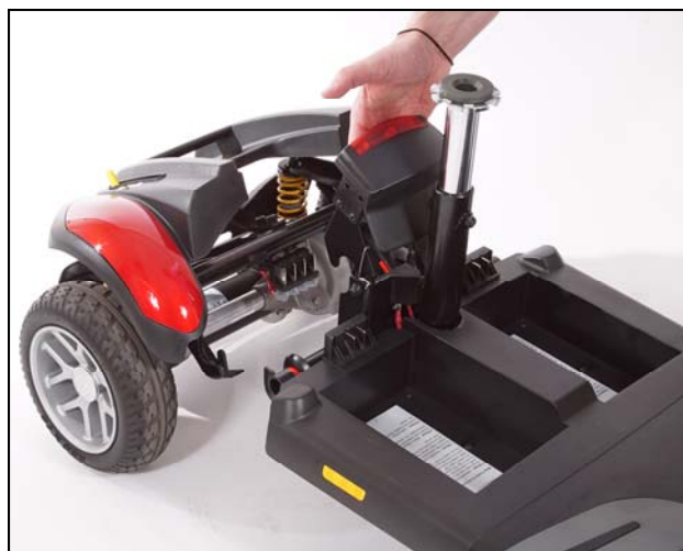
Figure 17. Separating the Drivetrain and Frame
