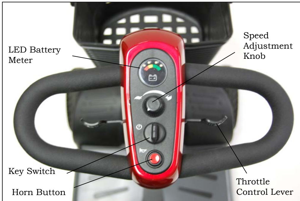
Figure 5. Buzzaround Extreme™ Delta Tiller Control Panel
