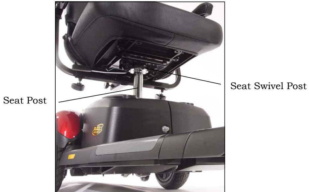
Figure 23. Installing the Seat
