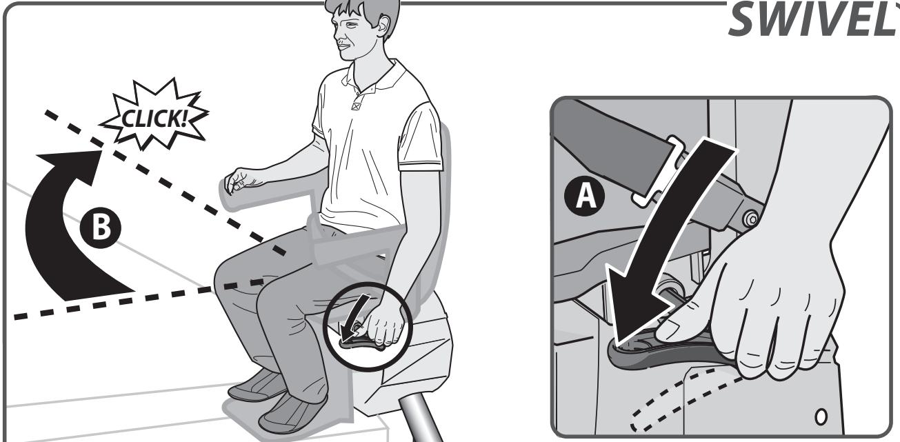
The lift stops automatically at the end of the rail. You can now swivel the seat manually, making it easier to get on and off. To do this, push down the lever{A}. Swivel the seat until you hear a 'click'. The seat is now in the correct position{B}.
