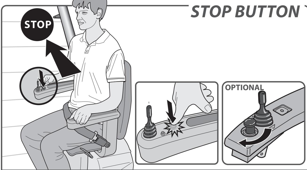
In an emergency, press the stop button once. The lift stops straight away. To release the lift, press the stop button again.
